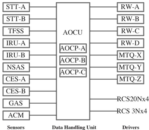
Figure 2.2.2: Block diagram of the *AKARI* attitude determination and control system.
