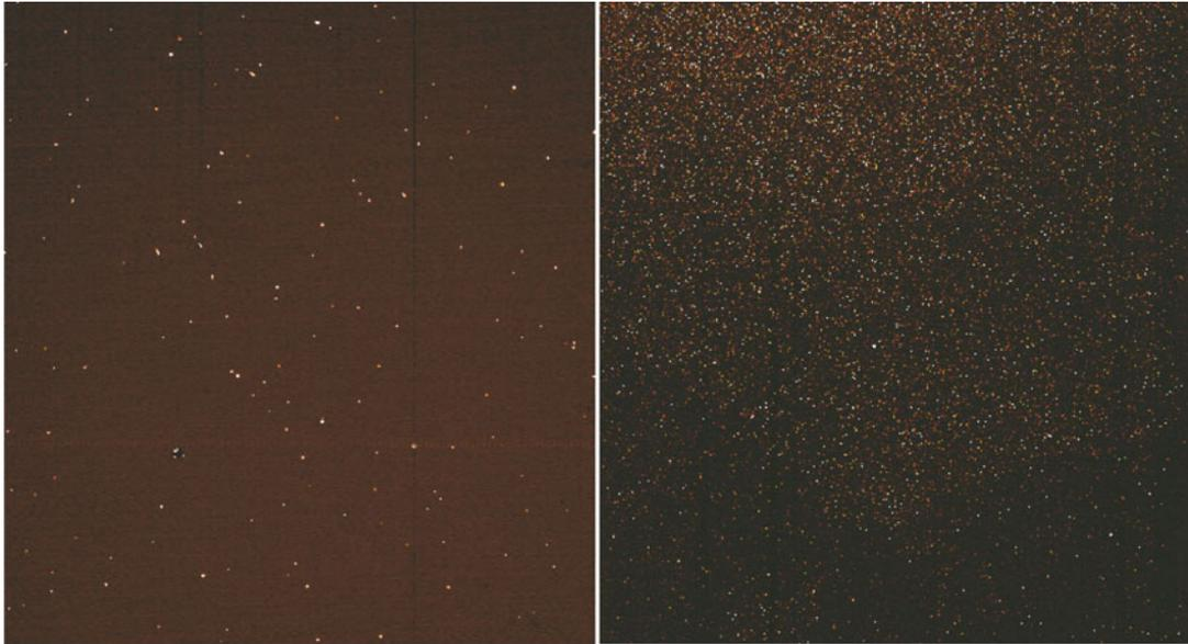
Figure 4.2.4: Dark frame images in phase 2 (a) and phase 3 (b) in the same ADU scale.
