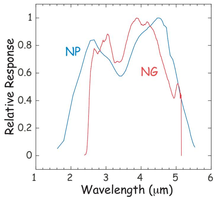
Figure 4.2.3: The Relative Spectral Response Function of the IRC/NIR dispersion elements per photon.
