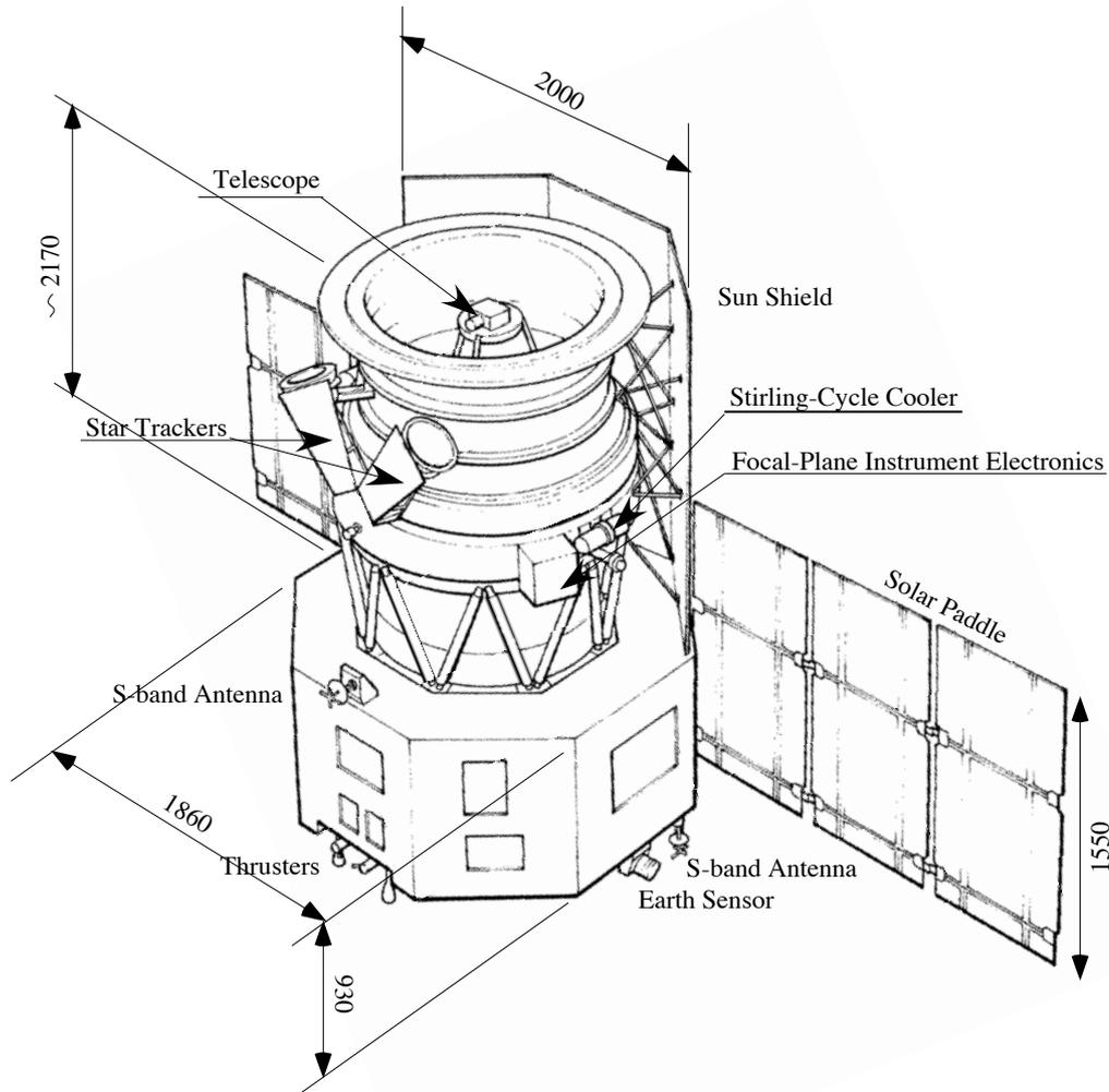
Figure 2.2.1: An overall view of the *AKARI* spacecraft (scales are in mm).
