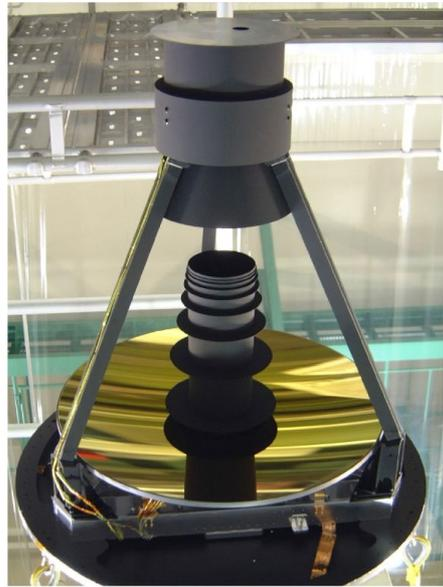
Figure 2.3.4: The *AKARI* telescope system.
