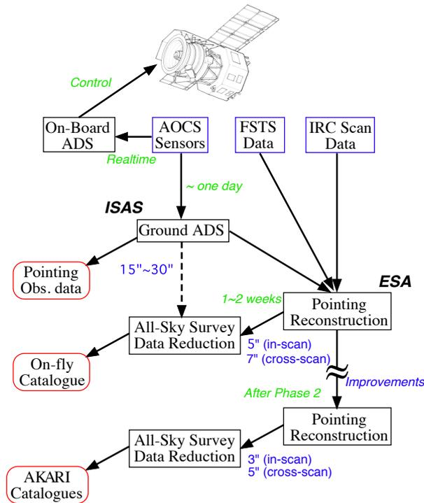
Figure 3.2.2: The outline of the *AKARI* attitude determination for the All-Sky Survey, including time scales and envisioned accuracy improvement. Note that the pointing reconstruction by ESA is not carried out for the pointed observations.
