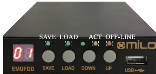
The AutoSave option has been added to simplify EMUFDD everyday's usage. When AutoSave is enabled, you don't need to manually save the current work before loading a new floppy or formatting a new one: EMUFDD automatically saves its internal memory to the current working floppy before loading/formatting.
