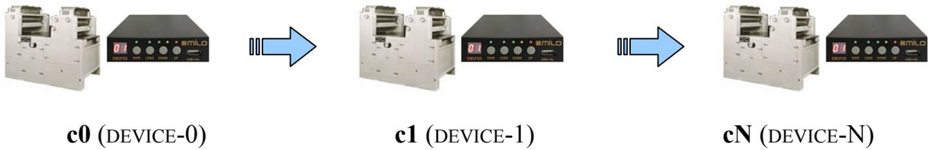
Connecting an EMUFDD “on-the-fly” it's very easy. You only need to modify, on each machinery, the floppy flat and power supply cables with longer ones, coming out from the machinery/control. After this modify, connecting/disconnecting the EMUFDD will be as easy as connecting/disconnecting a USB key and fast, since there's no more need to open the machinery to reach the floppy cables.
