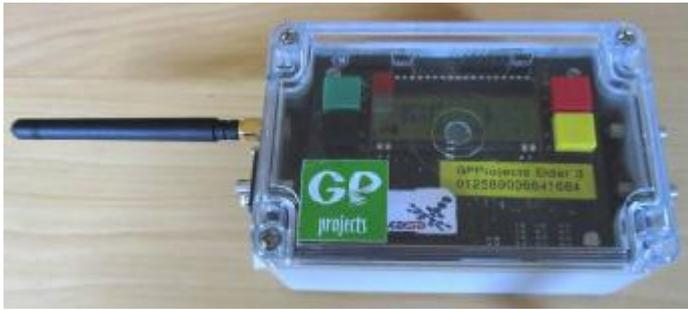
Punch data transmitted by an Eider unit is sent to the GPProjects servers, where it is stored in databases ready for viewing by results / commentary / safety software.
