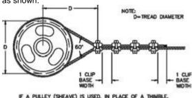
IF A PULLEY (SHEAVE) IS USED, IN PLACE OF A THINBLE, AND ONE ADDITIONAL CLIP. CLIP SPACING SHOULD BE AS SHOWN FIGURE 4.
