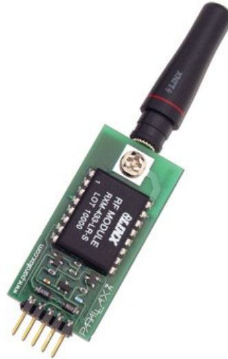
Illustration 7: RF receiving module.
