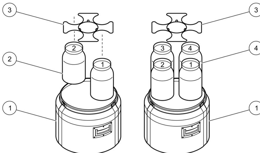
Figure 9 Two and four bottle installation
