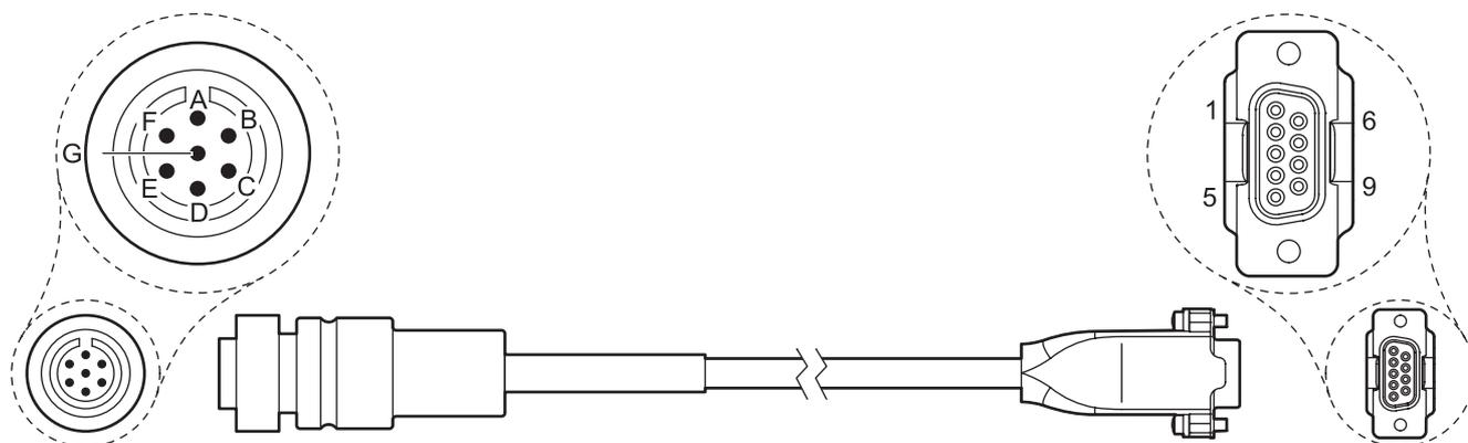
Figure 16 Serial connector cable
