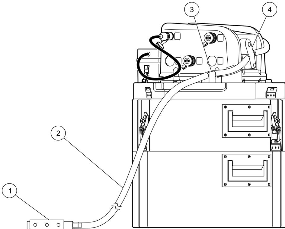
Figure 13 Intake tubing installation
