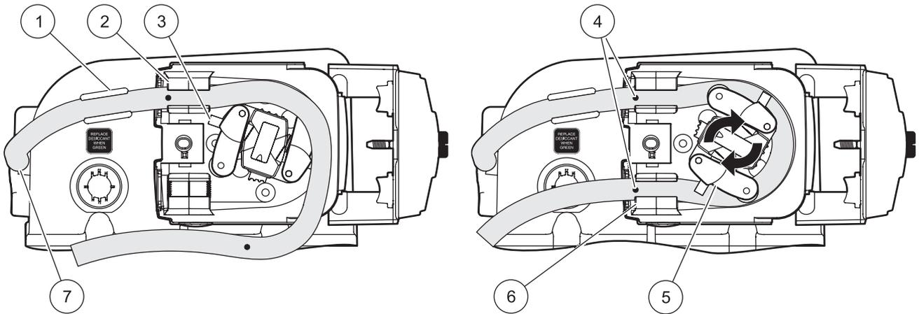
Figure 25 Pump tubing installation
