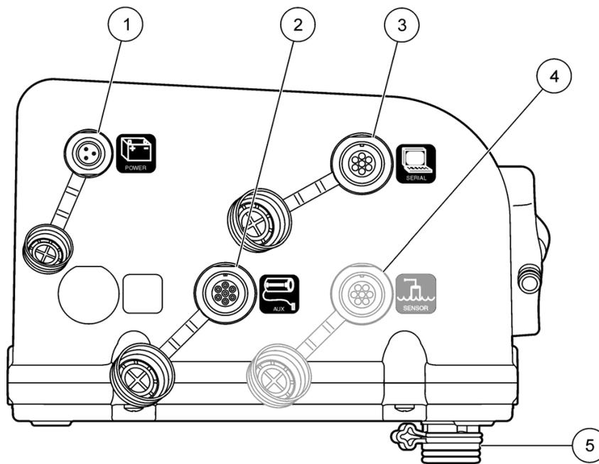
Figure 14 Side view of controller—connectors
