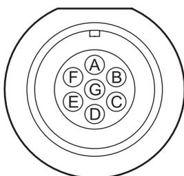
Figure 31 Auxiliary connector (7-pin)
