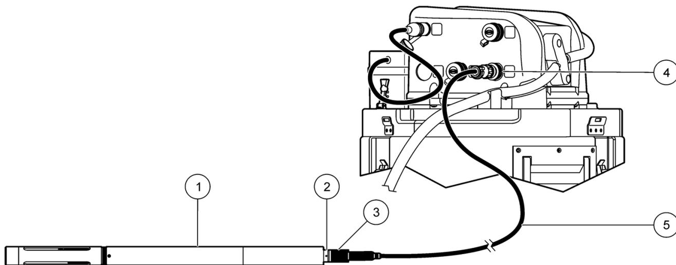
Figure 17 Sonde Connection
