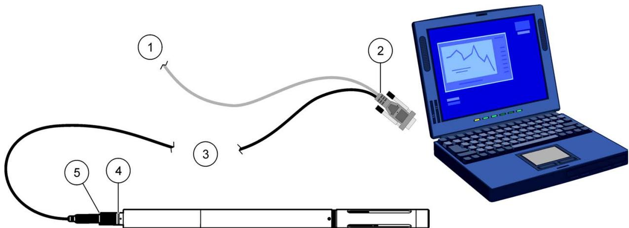
Figure 32 Setup for sonde with external power source
