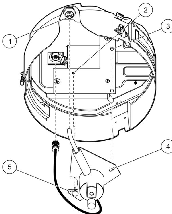
Figure 7 Full bottle shut-off installation
