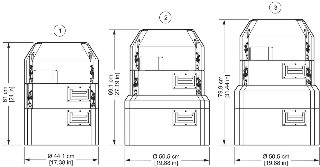
Figure 1 Portable sampler dimensions
