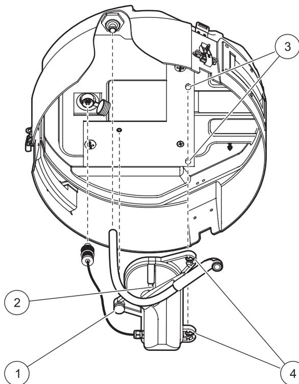
Figure 12 Distributor assembly installation
