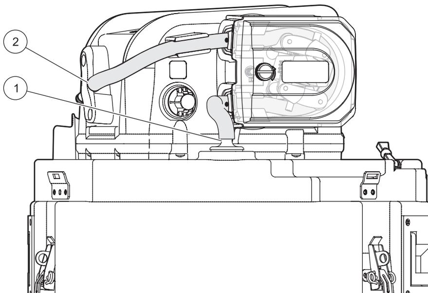
Figure 26 Pump tube installed
