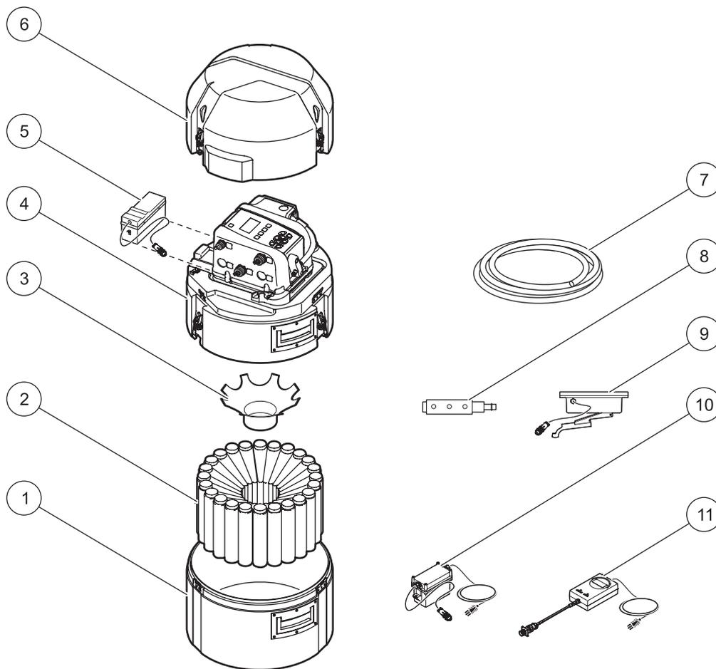
Figure 5 Sampler with multiple bottles
