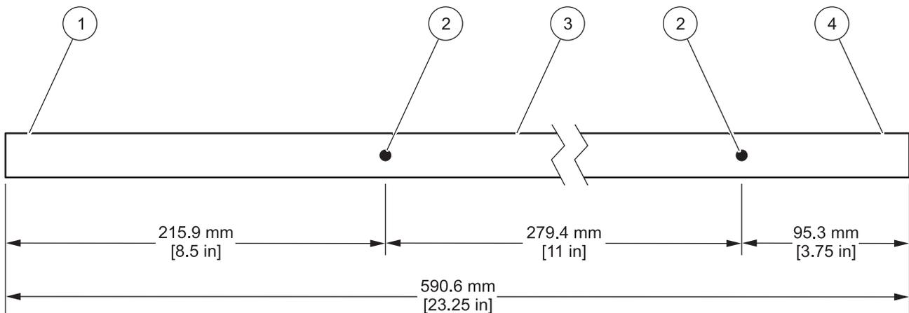
Figure 24 Pump tubing measurement
