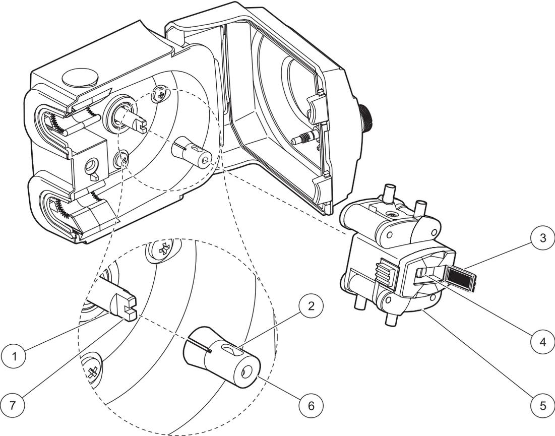
Figure 27 Pump rotor removal
