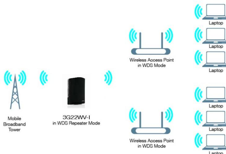
Figure 46: Advanced View - Wireless - WDS Repeater Mode
