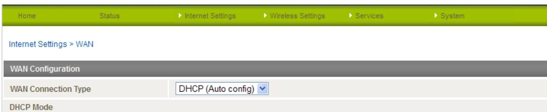
The screenshot shows the WAN Configuration page in the NetComm router's web interface. The breadcrumb trail is: Home > Status > Internet Settings > Wireless Settings > Services > System. The current page is 'Internet Settings > WAN'. Under the 'WAN Configuration' section, the 'WAN Connection Type' is set to 'DHCP (Auto config)'. Below this, there is a 'DHCP Mode' section with an empty input box.
