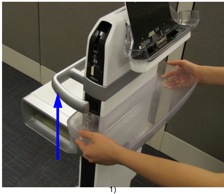
Figure 8-2 Docking Cart Plastic Shelf replacement
