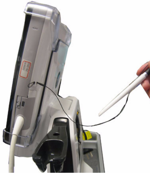
Figure 3-19 Connect stylus to Venue 40
