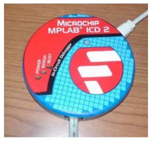
Go to the Microchip web page and read about the ICD-2 (in circuit debugger). You will use this device to program the PIC16F877. The debugger is about the size and shape of a hockey puck, and is pictured at the left. The debugger has three electrical cables connected to it: (1) a USB cable, which connects to your computer, a 9V power cable (not shown), and a 6-wire phone/data cable that connects to your circuit for programming.
