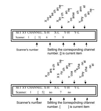
For 16Bit scanner, if the values of X-H,Y-H are set and the values of X-L,Y-L are set to [no], the 16Bit scanner will be running in 8Bit X/Y resolution. This will lost some characteristics of 16Bit scanner, such as high precision of X/Y orientation and the smoothness of the moving trace.
