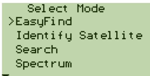
This is the Main Menu. Use the "**UP**"/"**DOWN**" buttons to scroll up and down in the menu system. Use the "**OK**" button to choose the selected function.
