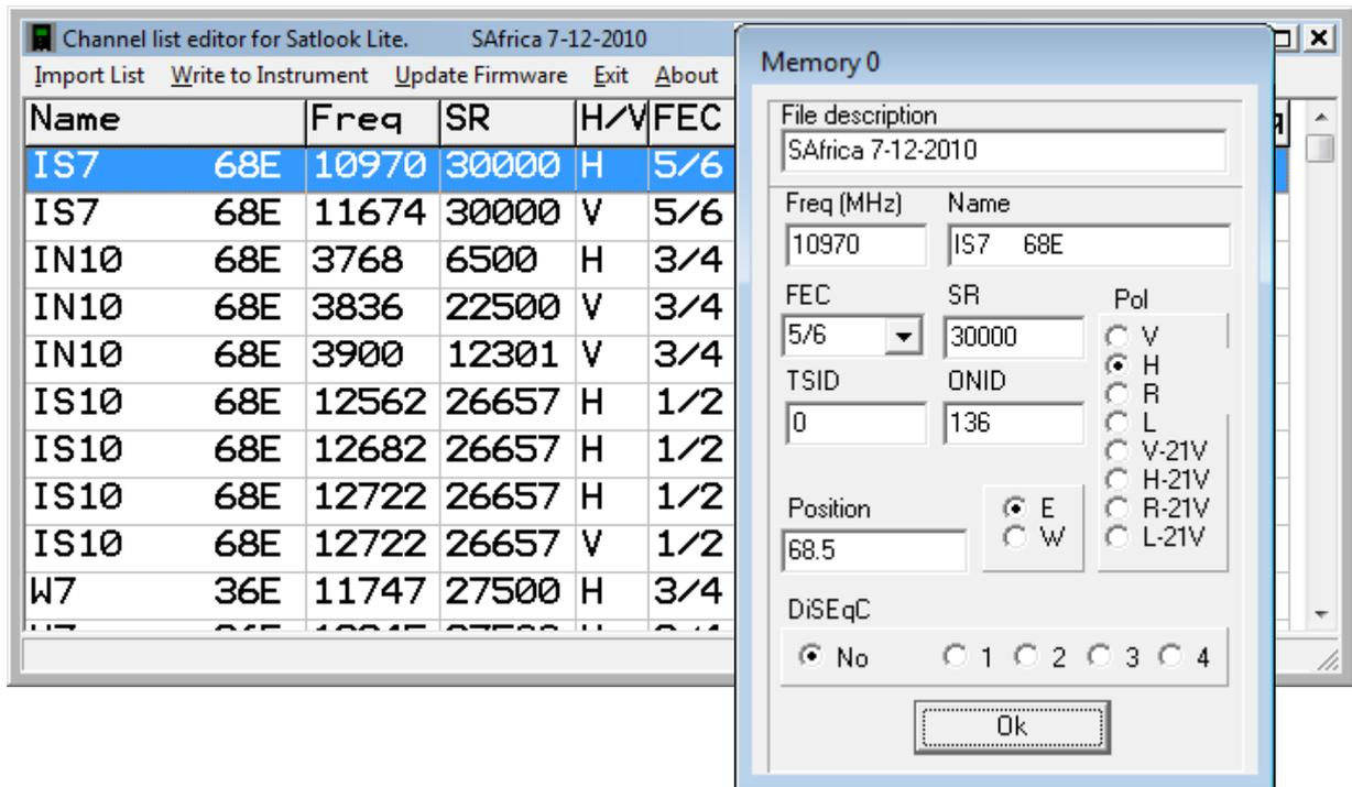
Clicking on a name allows editing the details for this entry. The “satlist.lst” files are stored as \*.csv files with the details below for each line.
