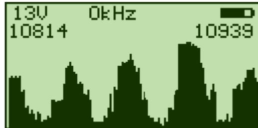
On entry, the spectrum display shows a 125MHz band centered on the current EasyFind satellite.
