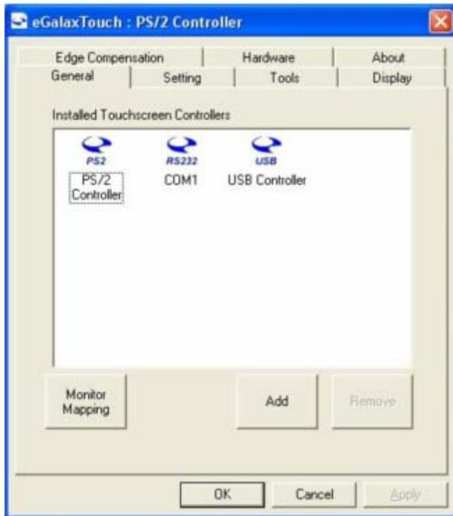
User can select the controller list in the window to do configuration for it. When user use a mouse or other input device to select the controller device in the controller list window, The controller name will be shown in the title bar of the main window( the property sheet ). Also, all of the other property pages will be updated for this selected controller. In some application, user may in place edit and change the controller name for easy identification.
