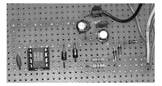
Fig. 2. Photograph of the temperature sensor board
