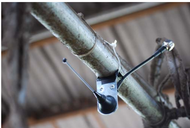
Fig. 15: Insulated mounting bracket fastened to an electrically conductive bar with insulating tape
