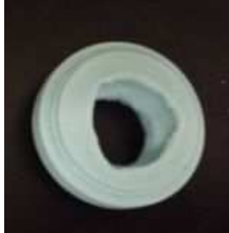
Figure 13. Example of holder moulded using a plaster replica of a surgical valve.
