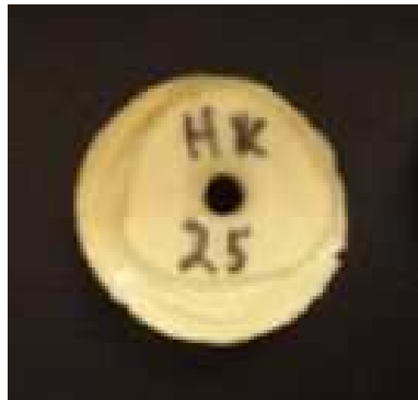
Figure 10. Complete plaster cast replica of valve, with centering hole for fastener.
