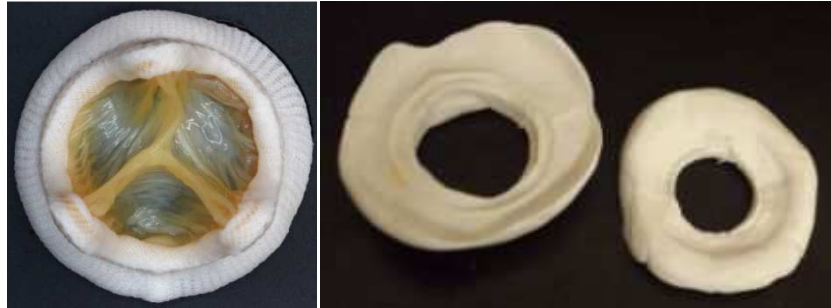
Figure 8. Putty impression (right) formed from Hancock II 505 CINCH valve (left).
