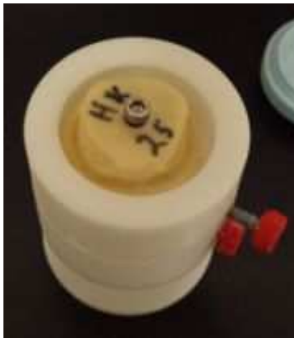
Figure 11. Valve replica mandrel fastened in holder mould.
