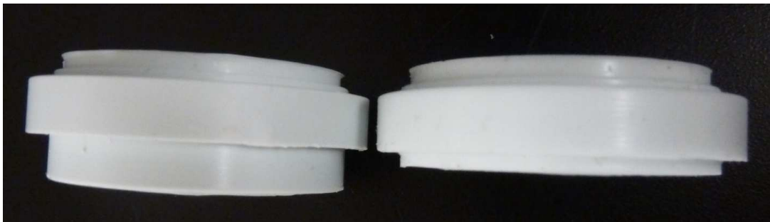
Figure 5. Device holders moulded without (left) and with (right) Insert E.
