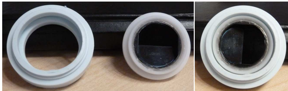
Figure 7. Carbomedics surgical mechanical valve sealed in Delrin™ fixture for interfacing with silicone holder.
