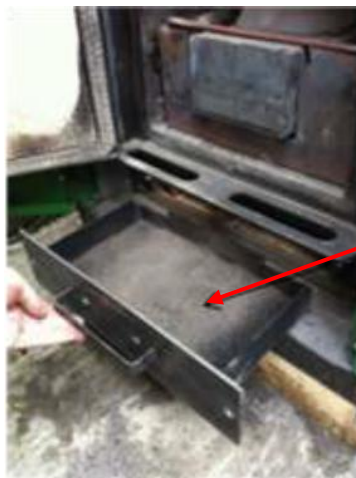
Carefully remove secondary ash pan and dispose of ash into a metal container.
