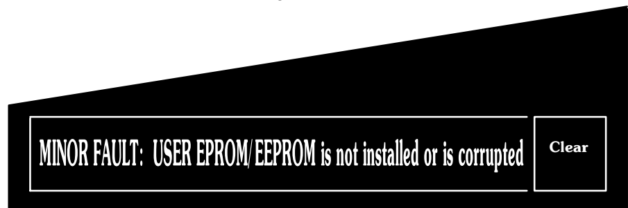
Figure 3 EPROM/EEPROM Minor Fault Message
