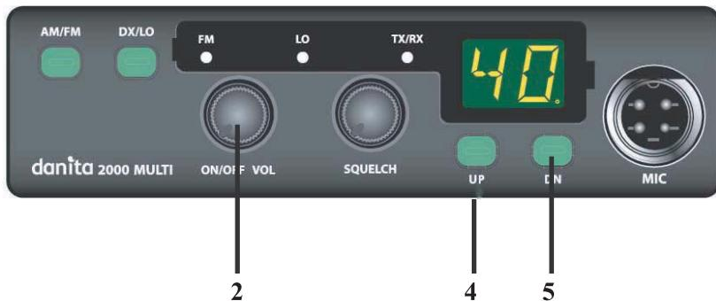
To change country selection, press UP knob “4” for 3 second, when danita 2000Multi is turned ON “2”. Select with UP/DN knobs “4+5”. Keep DN knob “5” pressed for 3 second for store new country.
