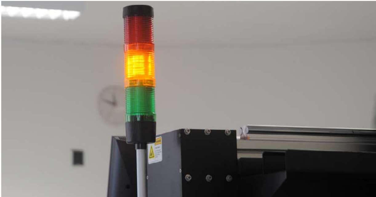
Beacon tower of lights. Not many printers have this system available.
