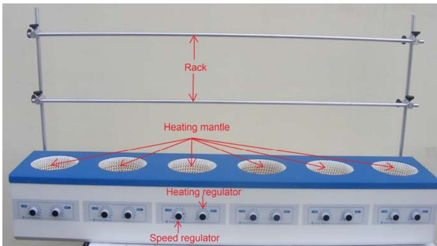
Stirrer indicator    Speed regulator    Heating regulator    Heater indicator
