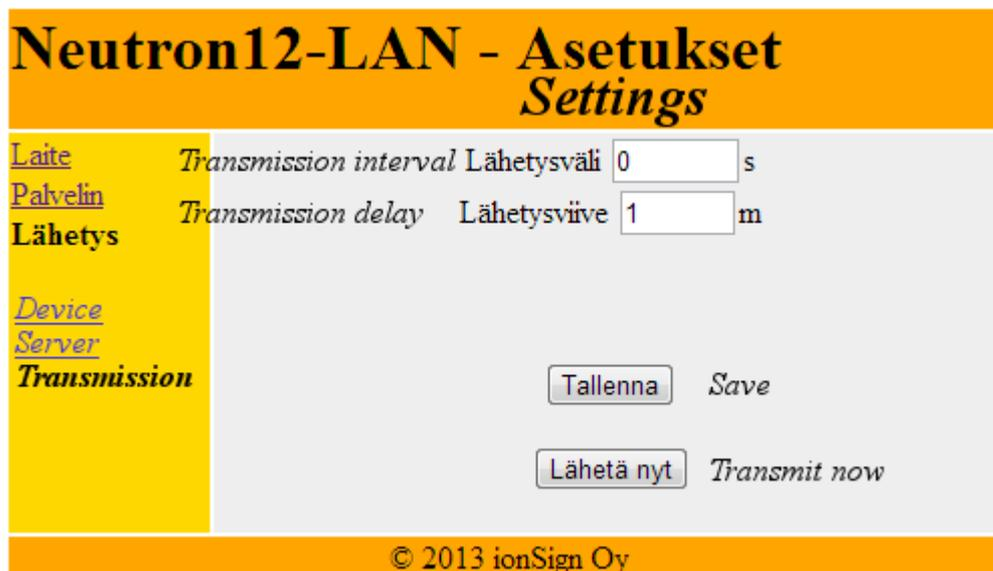
Picture 5: EXAMPLE – Transmission interval set to 0 s (only hourly data is transmitted at midnight) and transmission delay set to 1 min.
