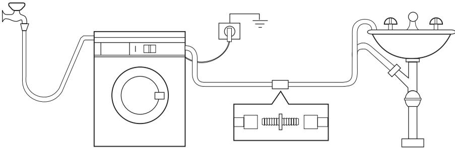
The drain hose may be extended to a maximum of 4 metres. An additional drain hose and joining piece is available from your local Service Centre.
