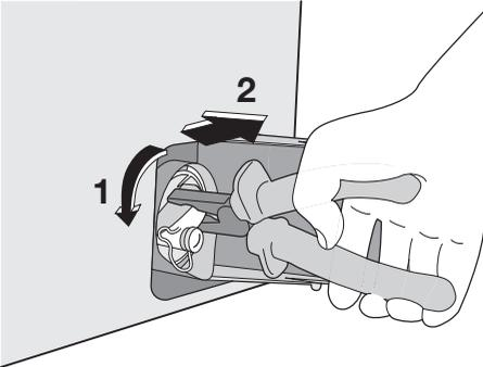
7. Remove any objects from the pump impeller by rotating it.
