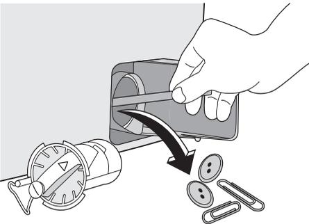
8. Replace the filter into the pump paying attention to insert it properly. When done, screw it firmly.
