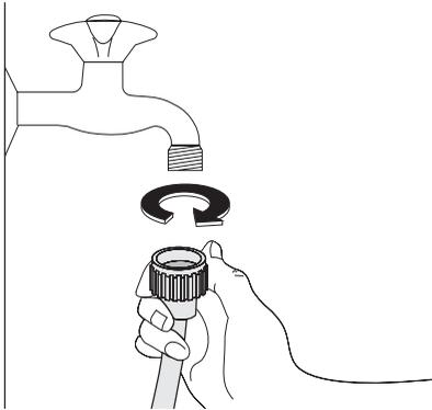
**Important!** Do not use the hose from your previous machine to connect to the water supply.
