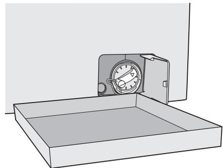
5. Pull out the emergency emptying cap from the filter cover, using a pliers.
