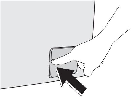
**Warning!** When the appliance is in use and depending on the programme selected there can be hot water in the pump. Never remove the pump cover during a wash cycle, always wait until the appliance has finished the cycle, and is empty. When replacing the cover, ensure it is securely re-tightened so as to stop leaks and young children being able to remove it.
