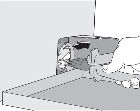
6. When no more water comes out, unscrew the pump cover, using a pliers, and remove the filter. Always keep a rag nearby to dry up spillage of water when removing the cover.
