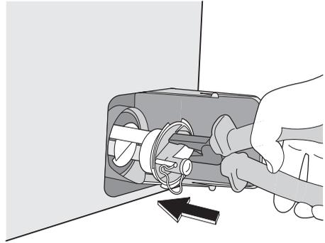
9. Replace the emergency emptying cap into the filter cover and fix it firmly.
