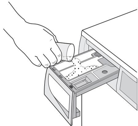
If required, pour fabric softener into the compartment marked
