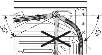
3. Set the hose correctly by loosening the ring nut. After positioning the inlet hose, be sure to tighten the ring nut again to prevent leaks.
