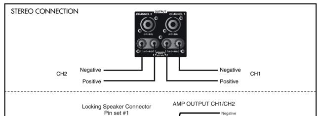
Stereo operation uses one positive and one negative terminal from the same channel.
