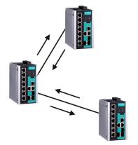
From the switch's web interface, you can enable or disable LLDP, and set the LLDP transmit interval. In addition, you can view each switch's neighbor-list, which is reported by its network neighbors. Most importantly, enabling the LLDP function allows Moxa's MXview to automatically display the network's topology and system setup details, such as VLAN and Trunking, for the entire network.
