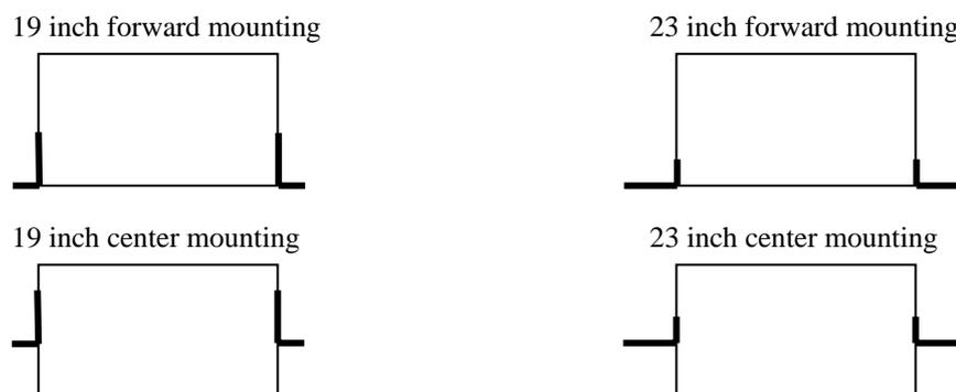
Figure 2-1 Chassis mounting options
