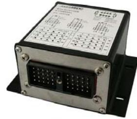
The RTD Scanner features rugged packaging and watertight Deutsch IPD connectors for an IP65 rating. The module is UL recognized for UL508 (FTPM2) – Controls for Stationary Engine Driven Assemblies and has a cUL recognition as well. The control carries a CE mark for the EMC and RoHS Directives. The AXRTD8 meets the environmental, EMC and vibration requirements of generator set applications in marine installations and has type approvals from several marine societies (LR, DNV, ABS, etc.).
