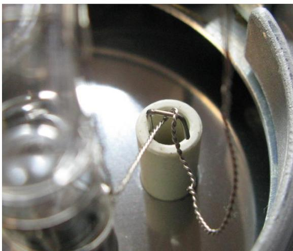
If the ignition wire is wrapped loosely onto the connecting pin the unit might not flash properly.
