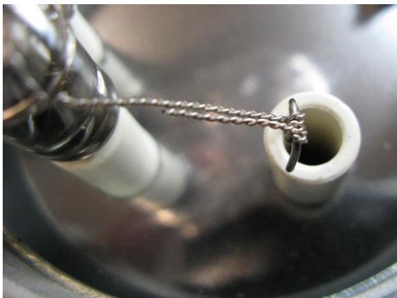
Wrap the ignition wire onto the connecting pin and afterwards onto itself facing the glass body.
