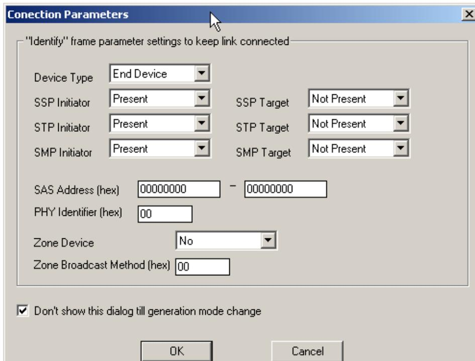
Figure 5.33: Connection Parameters Dialog
