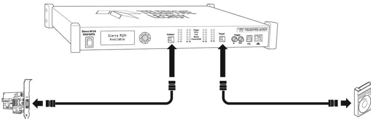
Figure 1.5: Analyzer MiniSAS HD Connections
