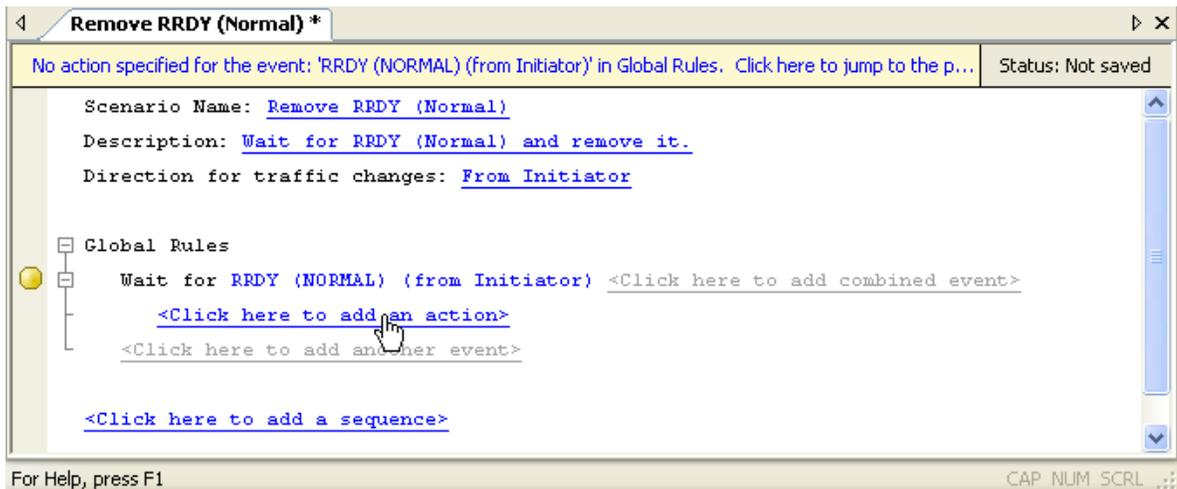
Figure 4.22: Example 1: Entering an Action
