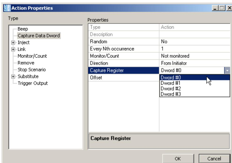
Figure 4.17: Capture Data DWORD Action
