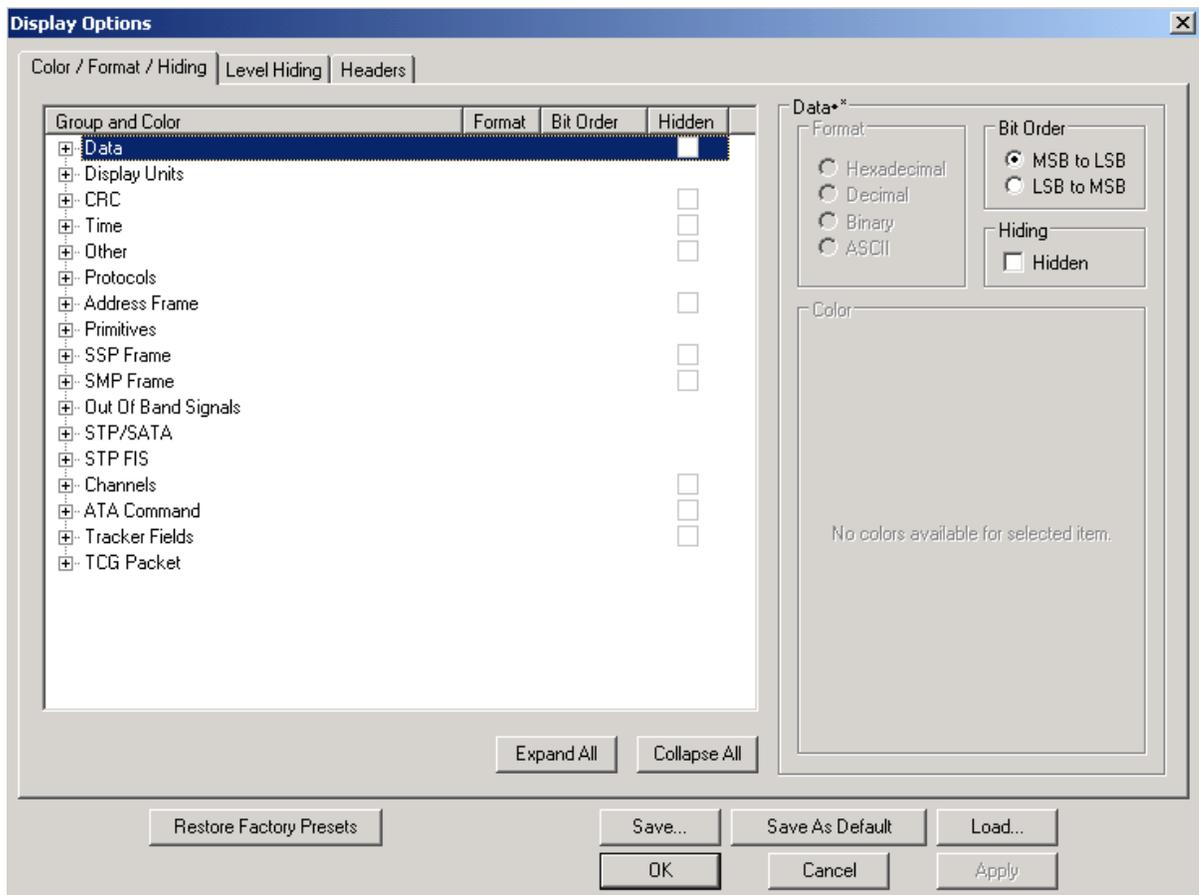
Figure 5.27: Display Options Dialog - Color, Format, Hiding Tab
