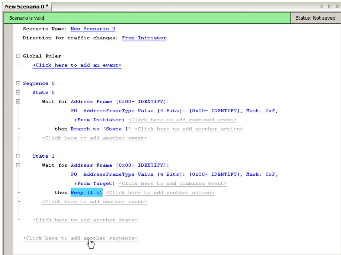
Figure 4.39: Example 7: Adding a Second Sequence
