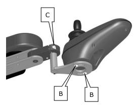
You can adjust the control unit to the inner or outer side.
