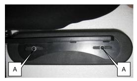
You can adjust the position of the armrest pad. Just unscrew the two screws (A) a bit and then you're able to shift the pad forward and backwards. After you reached the necessary position, tighten the screws (A) until the pad is fixed.
