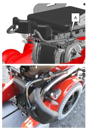
To use the knee support, make sure that it's adjusted correctly. Pull the quick release knob (A) and bring the knee support in position, release the quick release knob and make sure that it's locked in place. If the adjustments don't fulfill your requirements, please see chapter 8.7.2. to adjust the knee support. Adjustable knee pads are available.
