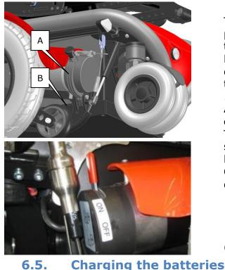
To disengage the motor brakes, to push the chair manually, switch off the control, pull the quick release knob (A) and press the lever (B) down respectively the lever from ON to OFF
