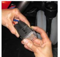
The main fuse housing is under the chair cover in the rear. To get access, carefully open the cover as shown above.
