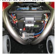
Open the fuse cover, insert the fuse which is delivered in a separate plastic bag and snap the fuse cover back. Now the chair can be brought into standing position to get access to the fuse cabling. Store the fuse cabling properly above the batteries and the main fuse housing below the control system under the chairs cover.
