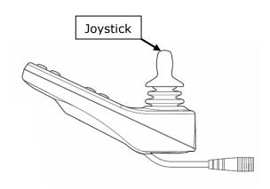
The joystick controls the direction and speed of the wheelchair.
