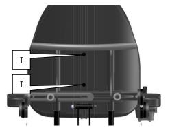
You can adjust the height of the backrest by untighten the two screws (I) a bit. Then you're able to shift the backrest up and down. If the backrest is in the desired position, tighten the screws (I).
