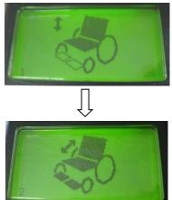
By pressing the MODE-button, you get into the standing function menu (picture A should appear on the display). If you now press the joystick forward, the seat is raising, if you press the joystick backwards, the seat is lowering. If your chair is equipped with the option "Tilt in space", you can choose this function in the standing menu
