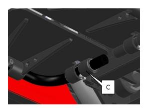
The angle of the footrest plate is adjustable by turning on the screw (C).
