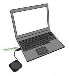
2. Place the activity monitor on the FlowLink with the display facing down. Make sure the **Align** light is lit on the FlowLink.
