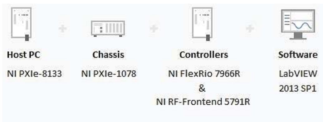
Figure 1: Content of the NI PXI system used for this radar application
