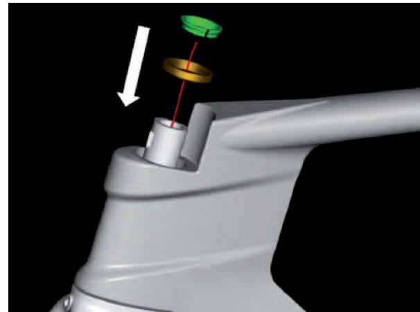
4. Route the brake cable through the front side steerer tube hole
