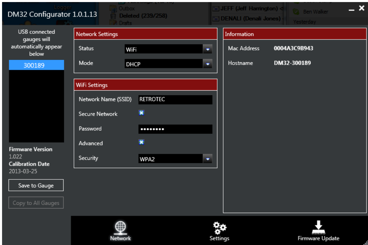
Figure 20: Some Secure WiFi networks need you to change the defaults in Advanced security settings
