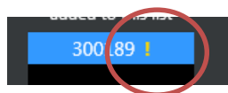
Figure 5: If a gauge has old firmware, the yellow ! will show up beside the serial number in the list
