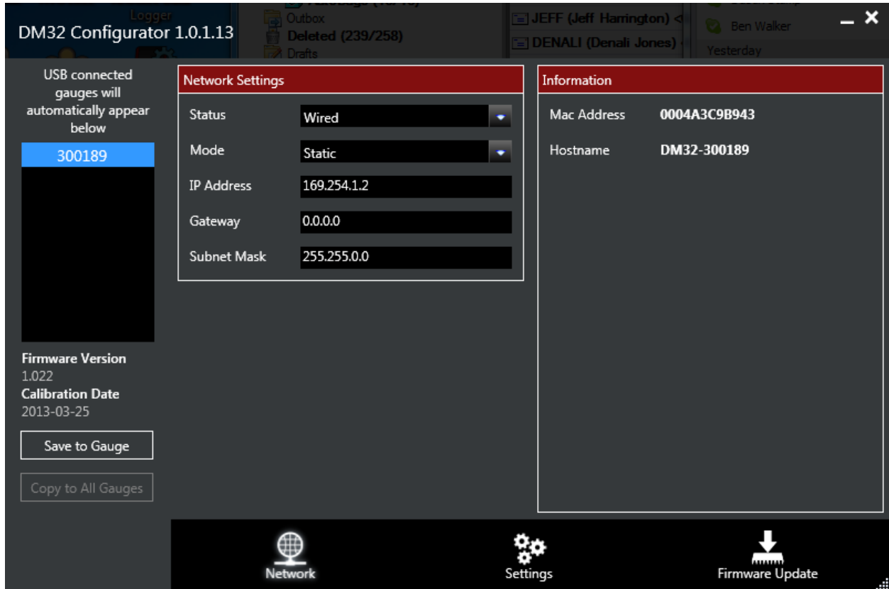
Figure 16: Wired network with a switch, hub, or direct to PC connection uses Static mode
