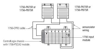
The 1756-PSCA2 chassis adapter module reduces horizontal space (on the right side of the chassis) when compared to a standard power supply, but increases vertical space (power supplies mounted above controller).
