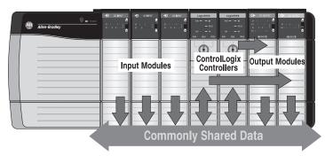
Each ControlLogix I/O module mounts in a ControlLogix chassis and **requires** either a removable terminal block (RTB) or a 1492 interface module (IFM) to connect all field-side wiring. RTBs and IFMs are not included with the I/O modules. They must be ordered separately.
