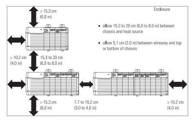
Enclosure 1756-PA75R or 1756-PA75R or 1756-PB75R 1756-PB75R 15.3 to 20 cm (6.0 to 8.0 in) 0 0 ControlLogix chassis È with 1756-PSCA2 module > 10.2 cm > 10.2 cm > 15.3 cm (4.0 in) (4.0 in) (6.0 in)
