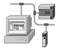
RSNetWorx software is the configuration tool for your control network. With RSNetWorx software you can create a graphical representation of your network configuration and configure the parameters that define your network.
