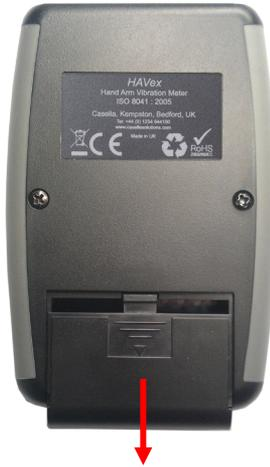
The cover can now be removed exposing the battery compartment and battery pack if fitted.
