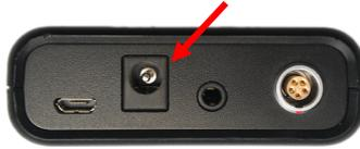
The HAVex instrument will not operate while the battery pack is charging and will immediately switch off when the charger is plugged in to the DC socket, even if the charger is not switched on. This is normal.
