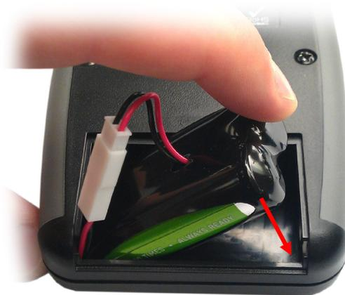
Push the raised end of the battery pack downwards as indicated until the battery pack sits comfortably in place.
