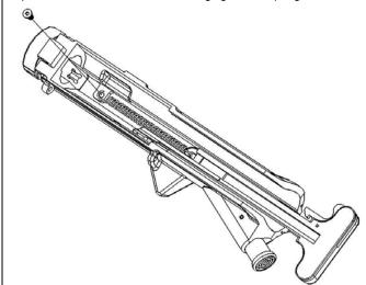
Step 06: Install outer barrel (not include)/ flash hider (not include)/ handguard (not include)
