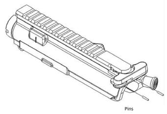
Step 03: Use screw to lock down charging handle spring.
