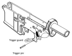
Step 08 : Use our trigger guard ping to install trigger guard (not include) Step 11 : We strongly suggest you to ask experienced Airsoft engineer to help you install the metal body.
