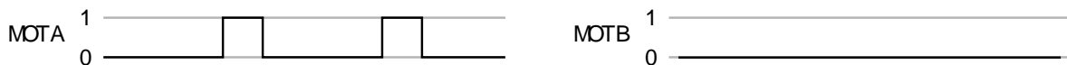
Figure 20: In this example, the motor will run in the opposite direction at around 25% speed.
