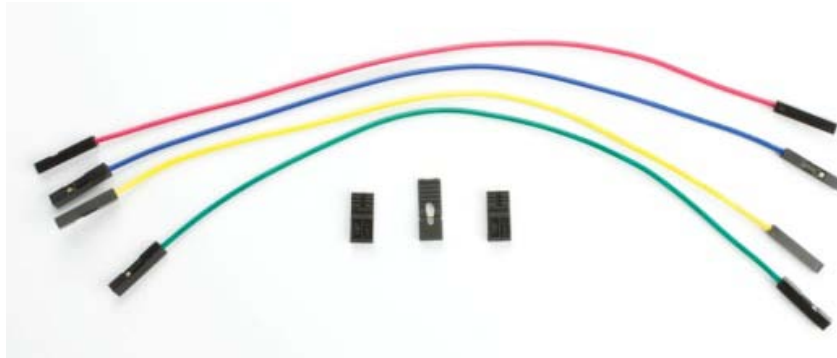
Figure 3: Photograph showing straps (the coloured wires) above, and jumpers below. Straps connect two parts of Gertboard together, whilst jumpers conveniently connect two adjacent pins together.
