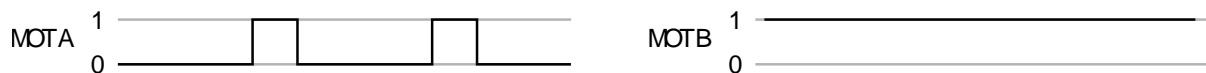
Figure 19: The motor direction is set by MOTB. Whilst MOTA has a duty cycle of 25%, the motor receives power whenever MOTA and MOTB are different, thus it receives power for 75% of the time.
