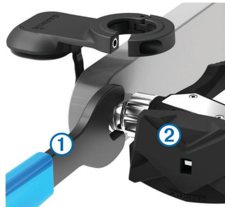
**NOTE:** The spindle and crank for the left pedal has a left-handed (reverse) thread.
