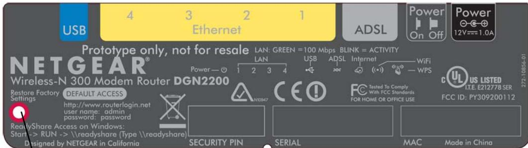
**Factory Default Reset.** Press for 6 seconds to reset the router to its factory default settings.
