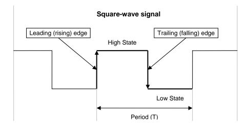
A **PULSE** is a signal whose amplitude deviates from zero for a short period of time. A pulse may be periodic (pulse train) and not periodic (single pulse). The **Pulse Width** is the time between the rising edge and the falling edge of a pulse. If the pulse is periodic it has a period and a duty cycle.
