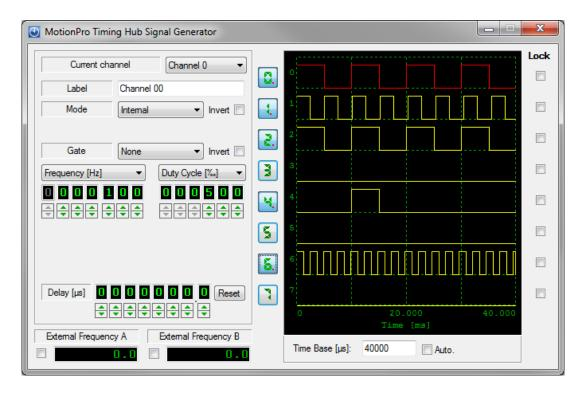
This application allows the user to generate signals with the timing hub. All the parameters of the timing hub may be changed. For each output channel, operation modes and delays may be set. The test program displays a dialog box with three areas.
