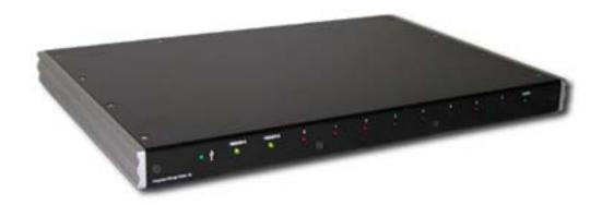
The **MotionPro Timing Hub** provides 8 independent synchronization signals, with 20 nanosecond resolution, to integrate different devices such as cameras with illumination. The CMOS level pulses are configured to operate in trigger, gate or burst mode. Each output can be clocked independently using an internally or externally generated source. The system is configured with two independent inputs for clock/trigger signals and provides continuous monitoring of their frequency and phase.
