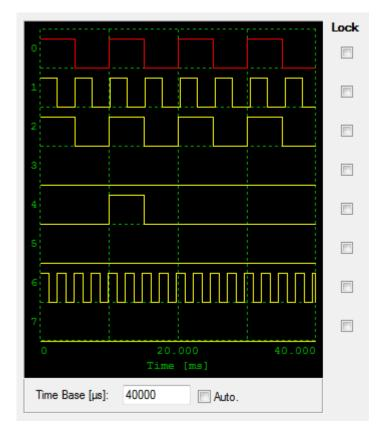
The output channels signals are shown in the black window. The user may select the Time base period. If the "Auto" option is selected, the application shows four periods.
