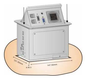
**Step3**: Secure the unit to the table : Take the support brackets under the table and place them into the support bracket grooves on both sides of the unit ; Verify proper alignment of the unit before tightening the mounting screws ; Screw both mounting butterfly screws upward until they reach the table ; surface (from underneath). Tighten firmly
