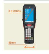
The 3.5 inch large screen and easy grip allow for high operability. In addition, frequently used keys such as the numeric keypad/ENT/SCAN are centrally located at the top to minimize finger movement, reducing fatigue.
