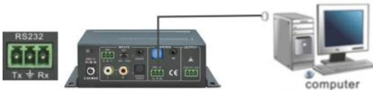
Figure 10 Connection of RS232 Port
