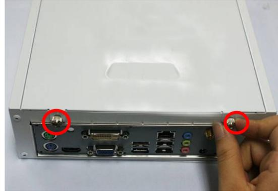
1. Slide the top cover into the chassis and put it in the direction towards the front panel (Make sure that the six metal hooks of the cover be fit into corresponding little slots in the chassis to make sure it firmly locked).
