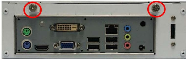
1. To remove the top cover from chassis, please remove the two screws on the back panel at first.
