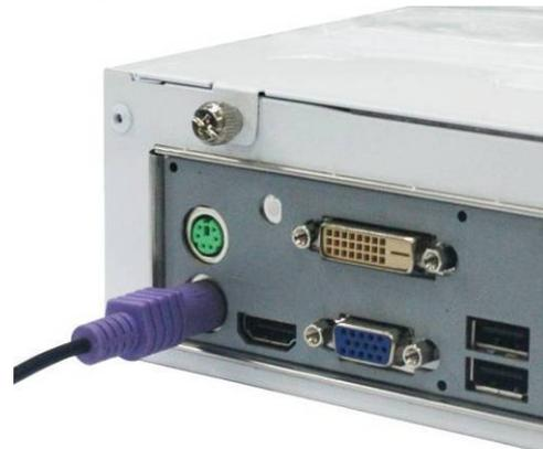
**PS/2 Keyboard Connector:** The connector is used for PS/2 keyboard connector.
