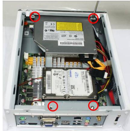
5. Lock the ODD/HDD bracket to the chassis by locking the screws in the marked places with a screwdriver.
