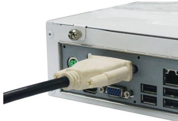
**DVI (Digital Visual Interface) Connector:** This interface standard designed to maximize the visual quality of digital display devices such as flat panel LCD computer displays and digital projectors.
