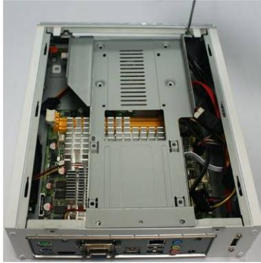
4. Remove the screws from the ODD/HDD bracket with a screwdriver.
