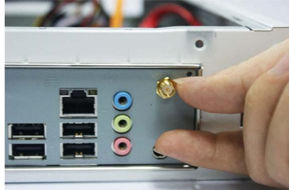
8. Fit the antenna connector into the RF slot from inside the chassis and then lock it into the panel by tightening another hexagonal bolt from the outside.
