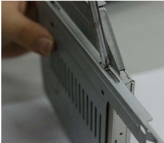
1. Install the optical drive disk to the appropriate position and then lock the screws with a screwdriver.
