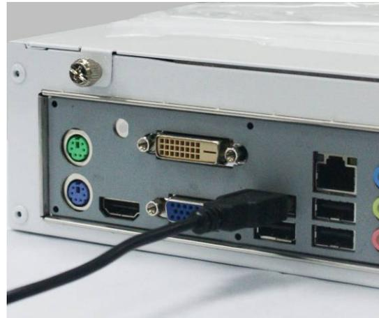
**USB Connectors:** There are 4 USB connectors on rear IO panel to connect USB mouse, keyboard and other USB devices to the system.
