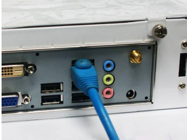
**RJ-45 Connector:** The connector is standard RJ-45 connector for Network. Please connect to the network cable to this connector.
