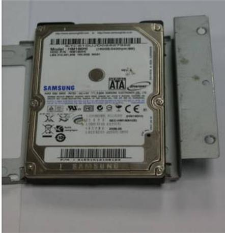
2. Put the 2.5 inch SATA HDD on the bracket with this side up.
