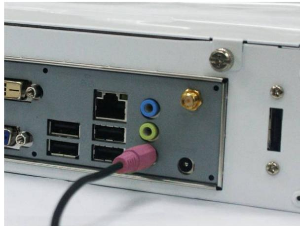
**Mic-In Connector:** User can connect microphone to this port.
