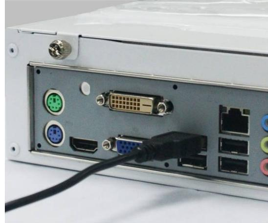
**HDMI (High-Definition Multimedia Interface) Connector:** This point-to-point interface is for audio and video signals designed as a single-cable solution for home theater and consumer electronics equipment.
