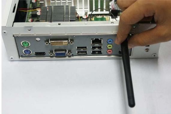
9. Connect the external WIFI receiver to the antenna connector on the rear panel.
