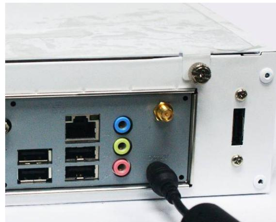
**DC12V Jack:** Connect the power adapter to DC12V jack after connecting connector power cord to adapter. Then Turn on the system either by power switch on front panel or remote control when all necessary configuration are made.
