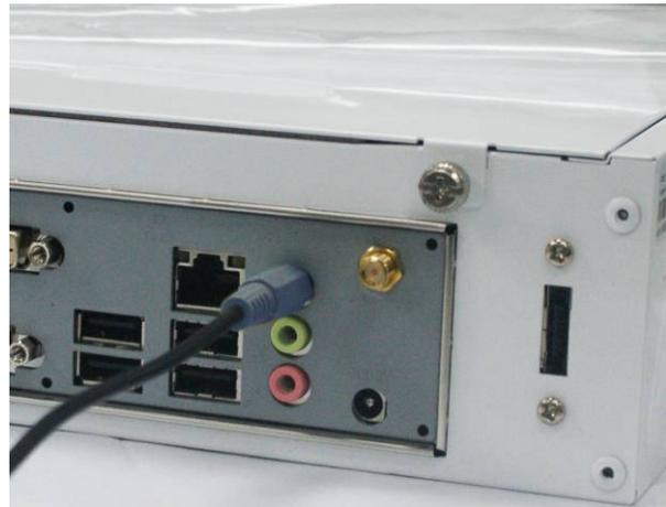
**Line-In:** This is a line-in connector for user to connect external audio device.
