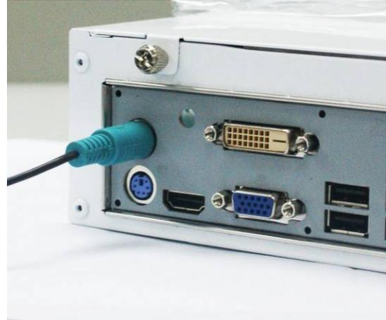
**PS/2 Mouse Connector:** The connector is used for PS/2 mouse connector.
