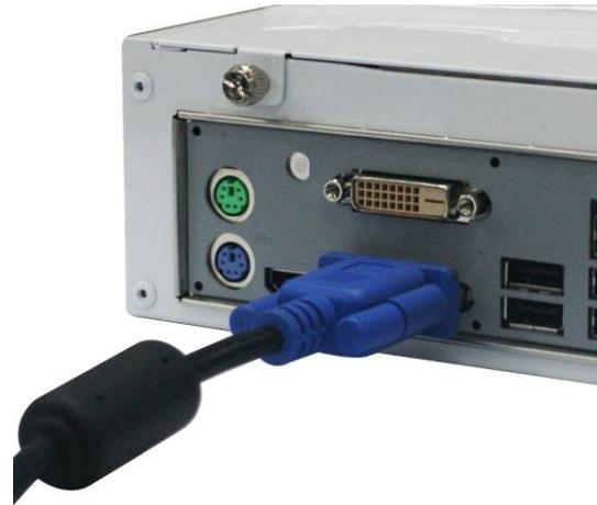
**VGA Connector:** VGA connector is the 15-pin D-sub female connector; it is for the display devices, such as the CRT monitor, LCD monitor and so on.
