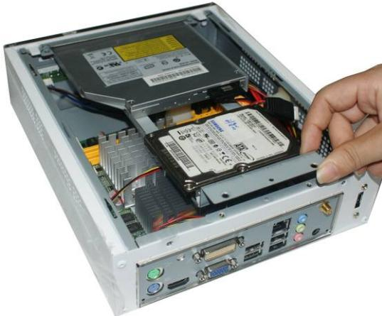
4. Pull the bracket with ODD and HDD locked with screws on it into the ODD/HDD bay.
