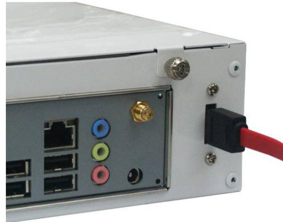
**E-SATA Connector:** Use E-SATA cable to connect E-SATA hard disk to the system.
