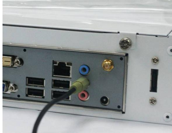
**Line-Out / Optical SPDIF out shared Connector:** Connect stereo speakers or headphones for audio output to connect Realtek 6-Channel HD Audio CODEC w/ SPDIF out audio output device for superior audio enjoyment.
