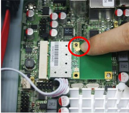
5. Press the metal hat on the other end of the antenna connector into the antenna slot (ANT1) on the mini-PCIE card as shown.
