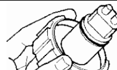
FIGURE 20 Remove and hold probe in the air to enter “0” for LOW setting.
