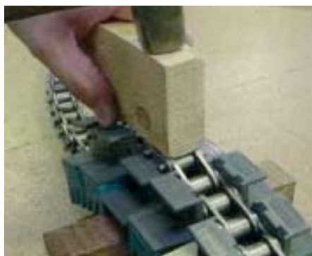
Picture 3: Assembling of the plastic plate Step 2: Assembling in the show way
