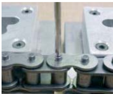
Picture 6: Cut the chain in the wished length Attention! use a compact base
