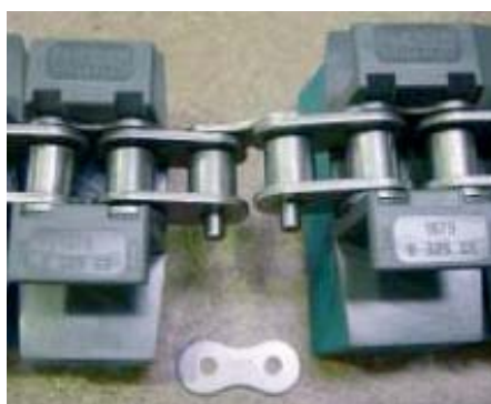
Picture 1: Connecting of two assembled chains with a connecting link
