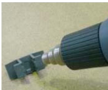
Picture 2: Assembling of the plastic plate. Step 1: heat to about 70° centigrade heating treatment time: 20 sec
