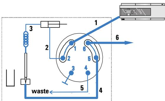
**Figure 3** Plumbing diagram (main pass)
