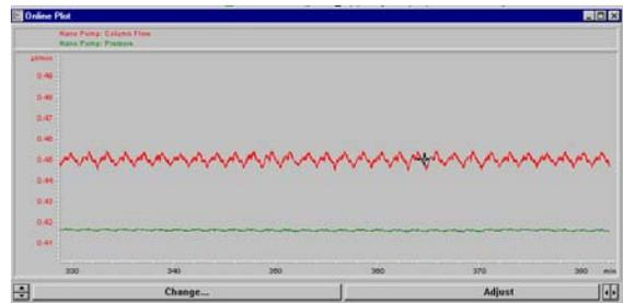
**Figure 4** Stability of flow (top) and pressure (bottom)
