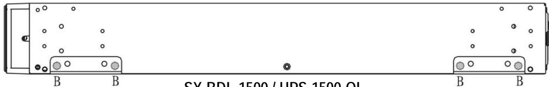
SX-BDL-1500 / UPS-1500-OL Use M5 x 12 screws on places marked with letter B
