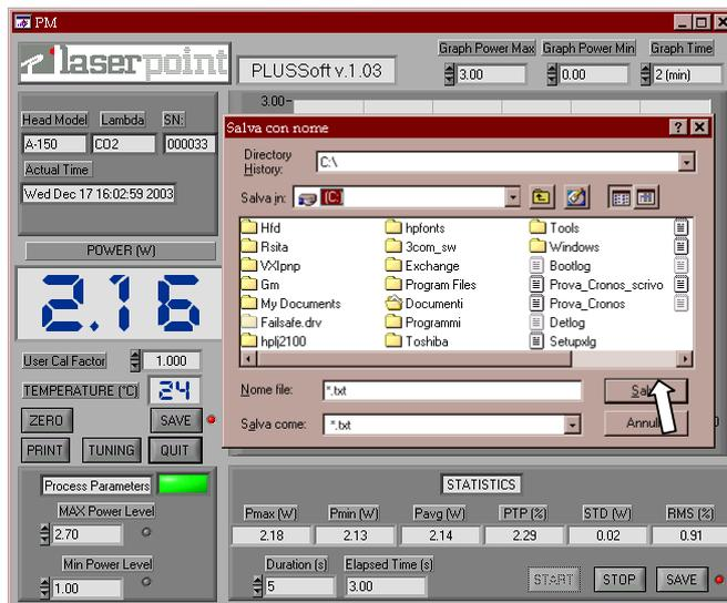
5. Select the folder on the *Save As* window and insert the file name. The Led will turn green. At the end of each Sampling Time the power value will be automatically saved
