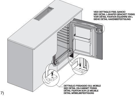
If the appliance has been installed correctly, when the cabinet door is closed it will be perfectly aligned with the adjacent units and the minibar's magnetic gasket will fit snugly against the edge of the front.
