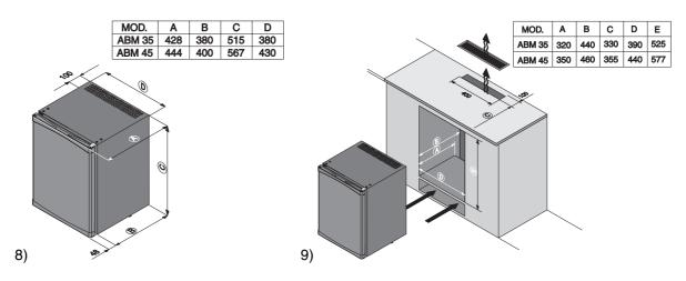
The area of both the air intakes and outlets must be at least 200  $\text{cm}^2$ .
